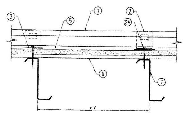
1. **Metal Roof Deck Panels\*** — No. 24 MSG min coated steel. Panels continuous over two or more spans. Endlaps to occur adjacent to purlin with panels overlapped 3 in. A bead of sealant may be used at panel end joints. ("Guardian II" only — Adjacent panels may be seamed with electric seamer with seaming operation to include roof deck fasteners (Item 2). Male/female side laps shall remain interlocked and fully engaged after seaming).
